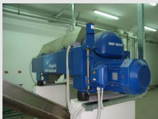
High-performance sludge dewatering centrifuge operating for up to 25 m 3 sludge per hour. The dewatering result is > 25 % dry substance.
