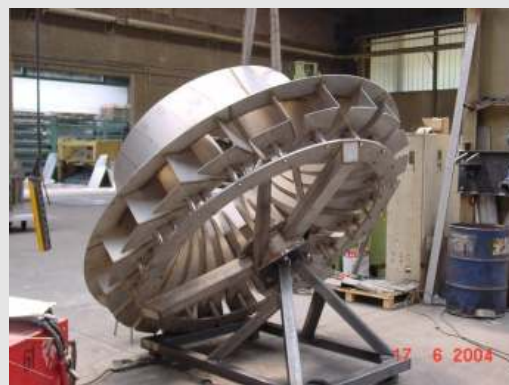
BSK®-surface aerator under manufacturing in the Biogest-workshop.
